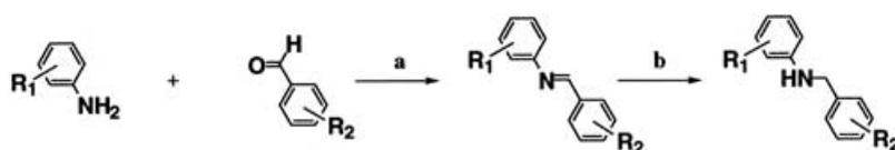
FIGURE 2 (a) Benzene, reflux (4h); (b) NaBH<sub>4</sub>, ethanol, reflux (2h).
